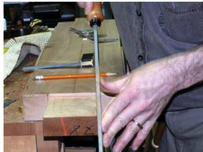
The flat face of the rasp is ideal for cleaning up the surfaces of many types of joints
