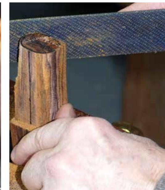
A coarse rasp quickly removes the hardest material, even this cocobolo
